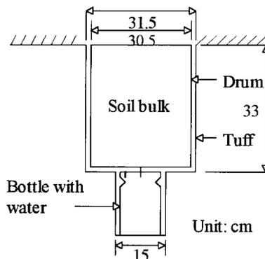
Figure 5. A schematic diagram illustrating the structure of the lysimeter and its settlement in the practical observations. [Modified from Figure 2 of Zhang *et al.* (1992)]
