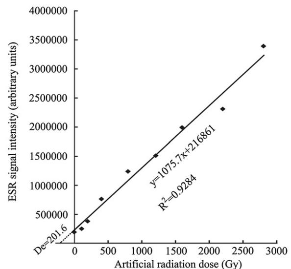
Fig. 5. Best-fit line between artificial radiation doses and ESR signal intensity (BGD-1-1).
