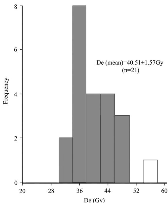
Fig. 6.  $D_e$ s histogram of the sample HG2-1. The empty column (aliquot with abnormal high dose) is excluded when calculating the average  $D_e$ .
