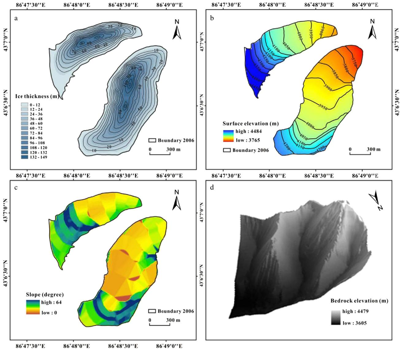
Figure 3. (a) Ice thickness and (b) the generated DEM from glacier surface topographic map of Urumqi Glacier No. 1 in 2006. (c) The glacier bedrock topography, constructed by subtracting the ice thickness from the glacier surface.
