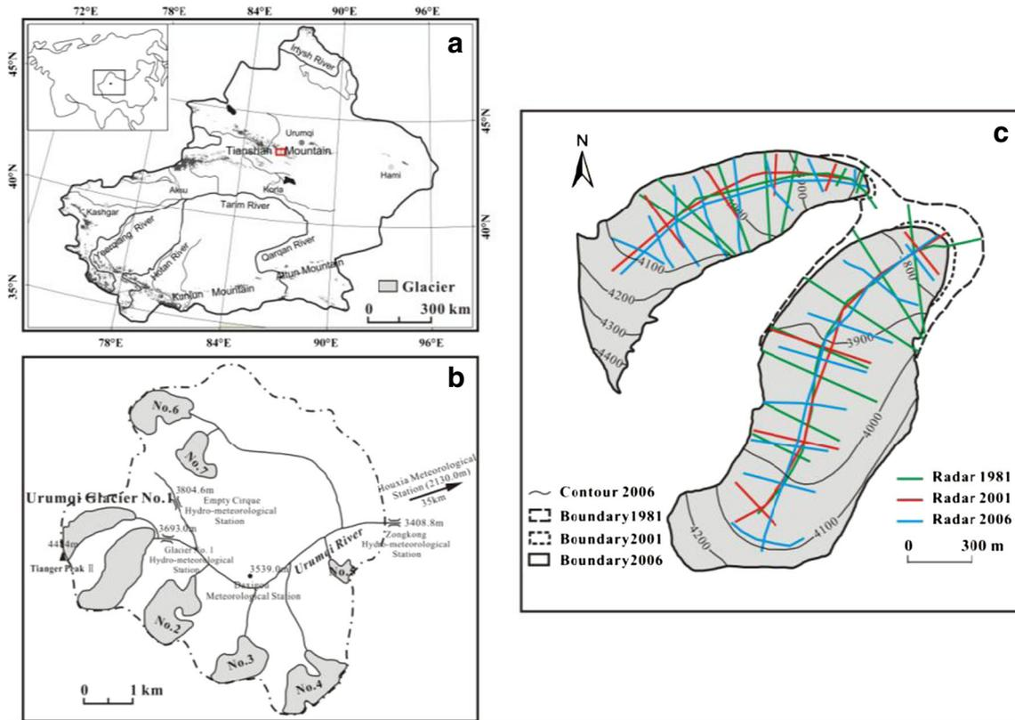
Figure 1. (a) Location of Urumqi Glacier No. 1 within the Chinese Tianshan, central Asia and (b) at the headwaters of Urumqi River. (c) The glacier surface topography, which is constructed by *in-situ* measurement in 2006. Contour interval is 100 m. The lines in different colours indicate the survey profiles of radar in 1981, 2001 and 2006, respectively. Glacier boundaries in different periods are denoted by different line types.
