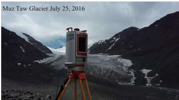
**Figure 2** TLS survey of Muz Taw Glacier in July 2016 with the Riegl VZ®-6000 terrestrial laser scanner
